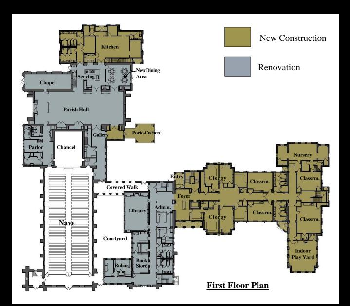
The main level plan with new construction in beige and renovated space in Gray.
